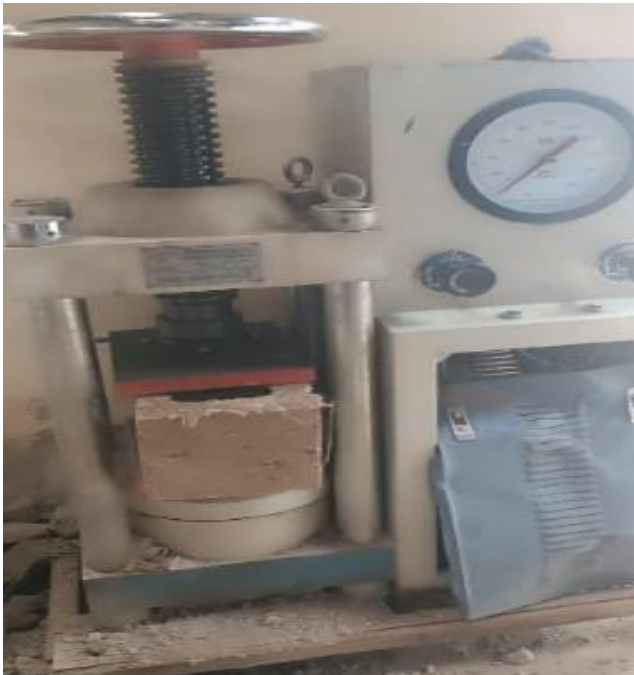
Figure 2. Compressive strength test
