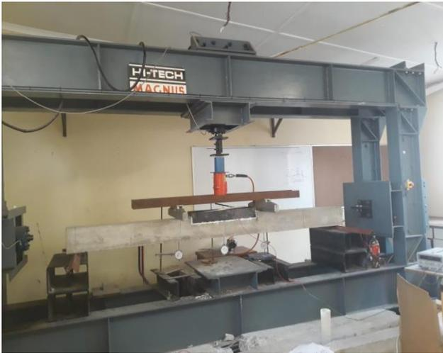
**Figure 3.** Pond placed and sealed at the center of the beam for accelerated corrosion.
