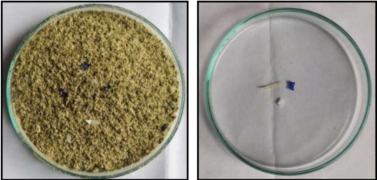
Figure 5 - Macroplastic particles were observed in the few samples, which were separated during the process of sieving
