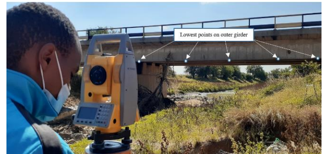
Figure 3. Bridge data collection using the Hi-Target total station
