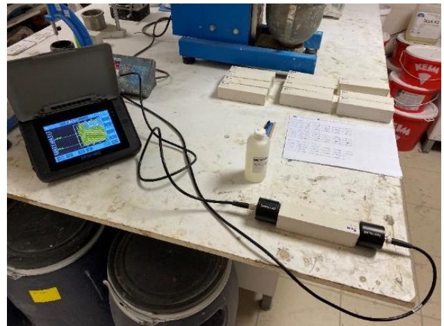
Figure 10. Application of the ultrasonic pulse velocity test.
