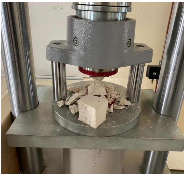
Figure 12. Compressive strength test setup.
