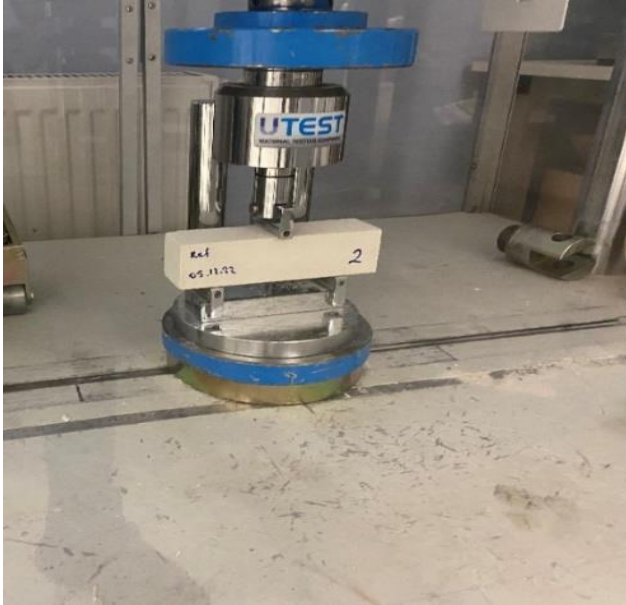
Figure 11. Flexural strength test setup.
