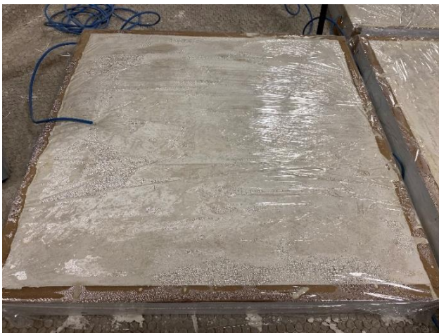
Figure 7. Concrete mixes placed in molds and covered with plastic wrap.
