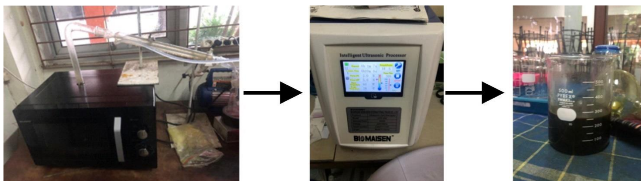
Figure 1. The process of extracting a nano liquid of the feed additive used was a combination of Andrographis paniculata and Moringa , and microwave-assisted extraction (MAE) was performed at a temperature of 50-60°C for 15 minutes. Nanoparticle-based extraction was conducted via ultrasonic-assisted extraction (UAE) for 10 minutes, which was repeated three times, for a total of 30 minutes.
