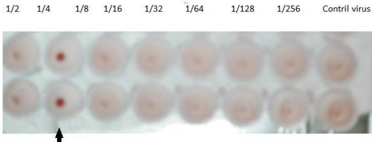
Figure 3. Inhibition of porcine red blood cell hemagglutination by chicken anti-CPV antibody. Inhibition of hemagglutination is indicated by settling porcine red blood cells at the bottom of a V-shaped microtitration plate (arrow).
